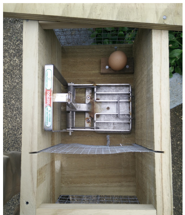
'Single set' DOC200 in box. The kill bar is down and the trap is unset.
